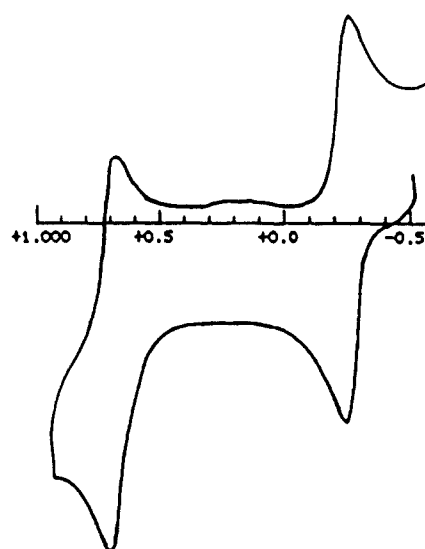
Figure 8. Cyclic voltammogram of \text{Co}_3(\eta^5\text{-C}_5\text{Me}_5)_3(\mu_3\text{-CO})(\mu_3\text{-NH}) (IIc) in \text{CH}_2\text{Cl}_2/0.1 \text{ M TBAPF}_6 at a platinum disk electrode with a scan rate of 100 \text{ mV/s} . Two reversible one-electron oxidations occur at E_{1/2} = -0.21 \text{ V} and E_{1/2} = +0.75 \text{ V} (vs. SCE).
